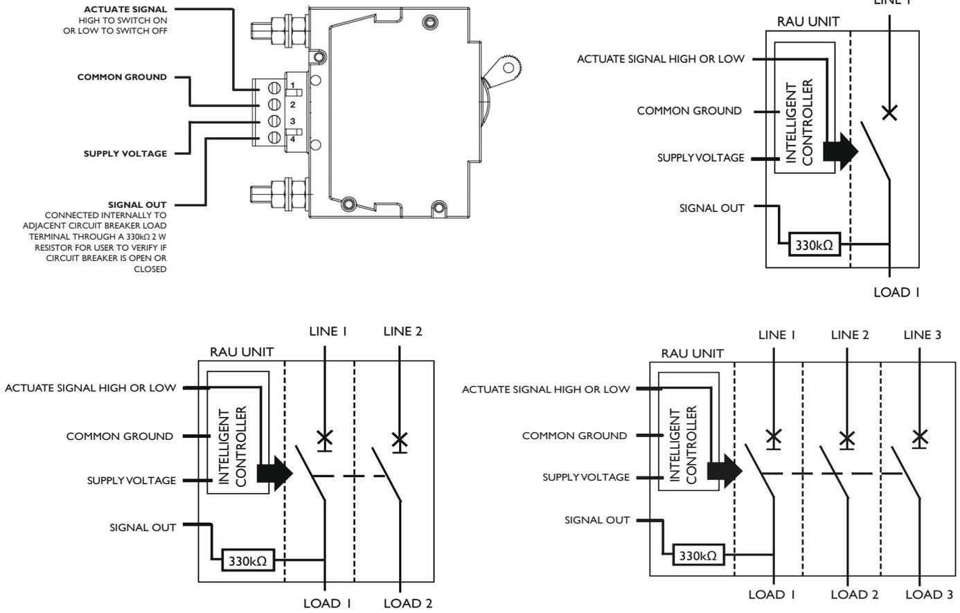
Note: Signal out only provides status indication of the adjacent pole through a 330 kΩ resistor.
