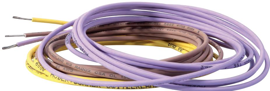
RADOX® 155 are flexible single core and multi core cables offering excellent resistance to heat, hot pressure and aging. The electronically crosslinked insulation offers high mechanical ruggedness. It will not melt and is resistant to most media as well as insulating varnishes and impregnating resins. Brief exposure to heat up to +280 °C will not have any lasting effect.
